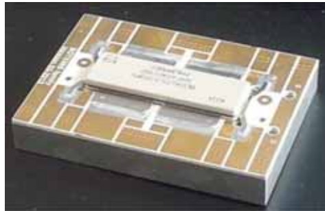
Fig 23. Example of soldered RF transistor in a demoboard
