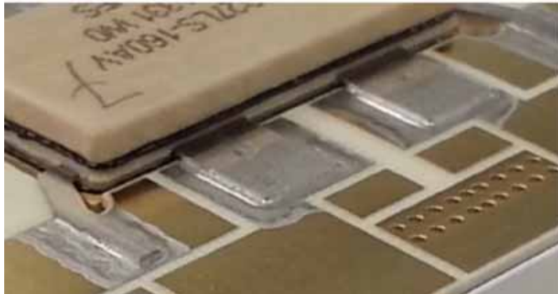
Fig 28. Wetting appearance (Pb-free solder joints)
